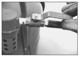
Figure 12. Tank air supply valve, opened.
